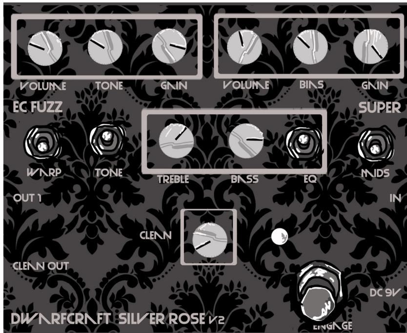
**VOLUME (left)** - Controls the volume of the EC FUZZ circuit
