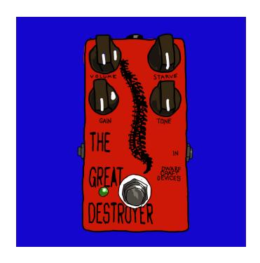
**DC JACK** - Plug in the 9v DC center negative plug here. Please use a high quality power supply, or risk this thing being even noisier. **IN** - Plug your 1/4 inch instrument cable in here
